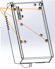
The evaporator can now be released by levering a small screwdriver through the two openings.
